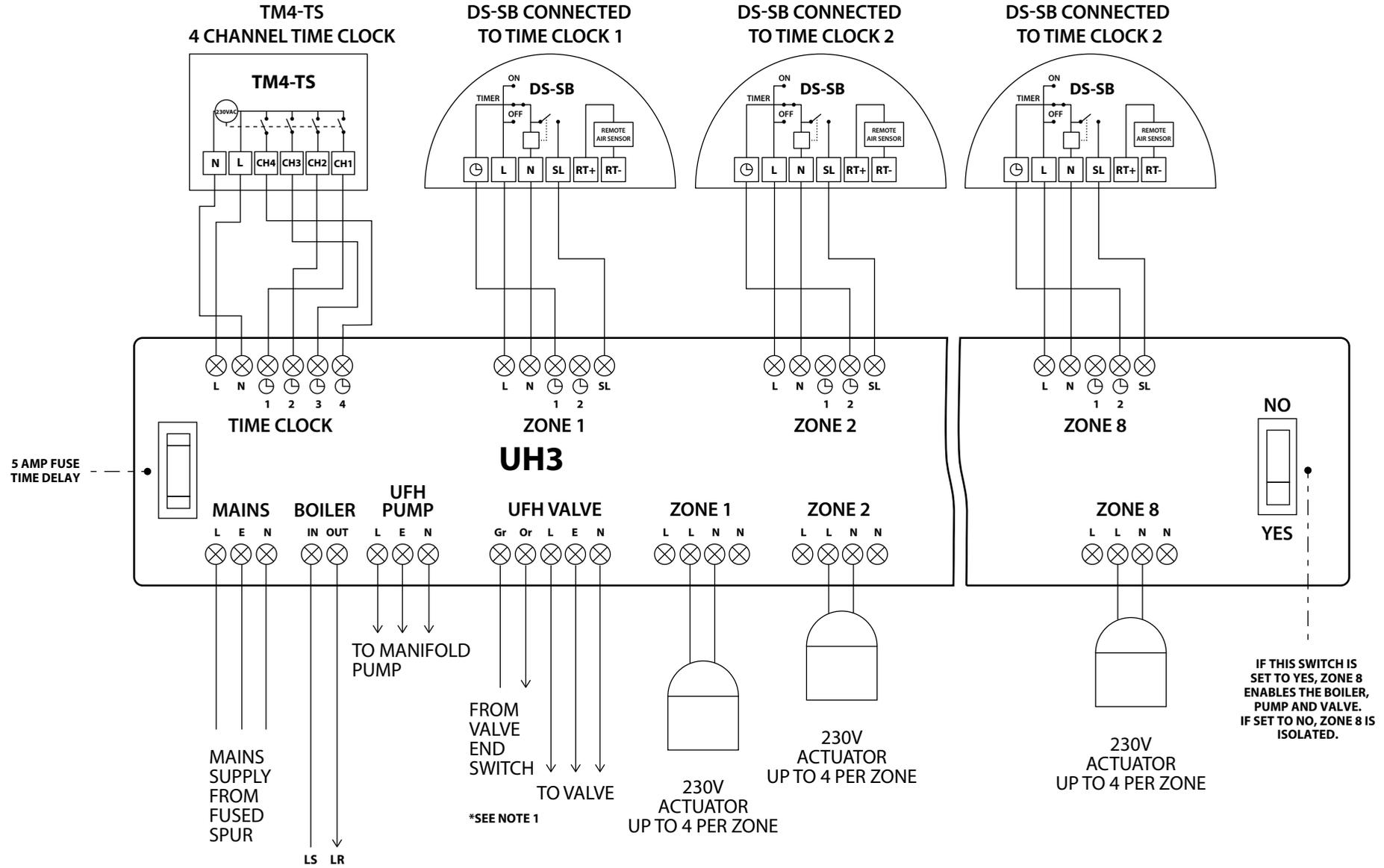
N.B. For boilers requiring a switched live signal connect LS to permanent live and LR to the boiler.
